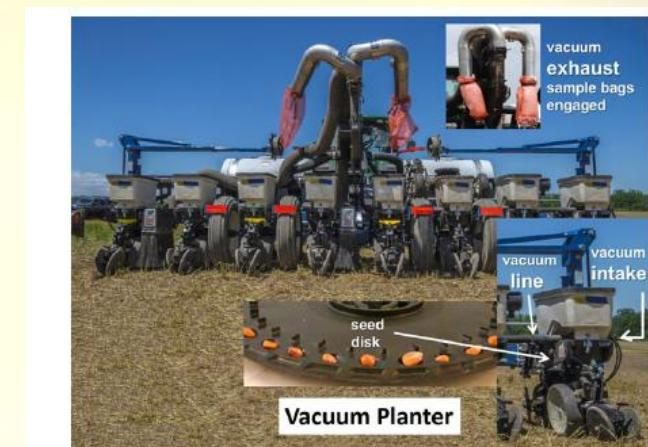
Figure 1. Kinze (Kearney Canada) vacuum planter showing exhaust location and dust collection device (top inset).
